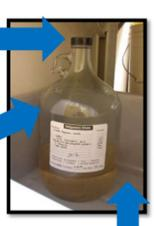
Keep waste container in a secondary containment bin.
